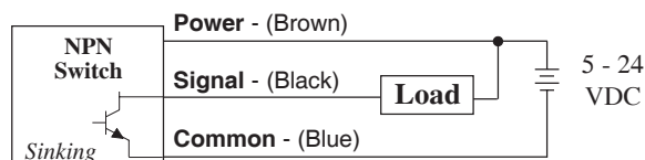
NPN wiring connection - both NC &amp; NO
