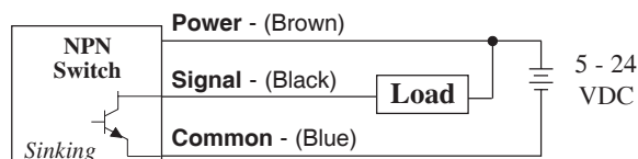
NPN wiring connection - both NC &amp; NO
